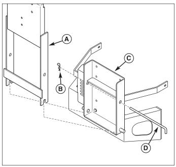
Figure 10. Install Back Plate (Flat Style Bumper shown)
